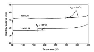
Fig. 5. Typical DSC thermograms of poly(ester amide) 4i (heating rate = 20 °C/min).
