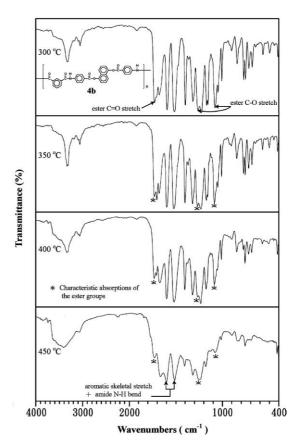
Fig. 8. FT-IR spectra (thin film) of poly(ester amide) **4b** after sequential heating in air at the indicated temperatures, each for 10 min.
