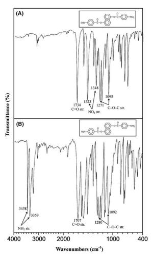
Fig. 1. FT-IR spectra of (A) dinitro-diester 1 and (B) bis(ester amine) 2.
