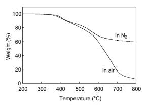
Fig. 7. TGA curves of poly(ester amide) **4c** (heating rate = 20 °C/min).
