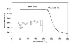
Fig. 6. Typical TMA thermogram of poly(ester amide) 4c (heating rate = 10 °C/min and applied force = 10 mN).
