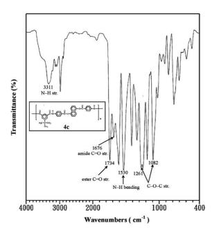
Fig. 3. The thin-film FT-IR spectrum of poly(ester amide) 4c.
